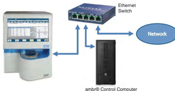
Figure 3.10 Option 2: FLEX2 and ambr® connected to lab network via Ethernet switch
