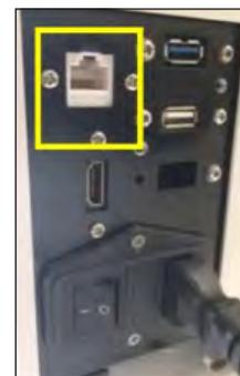
Figure 3.8 NIC on rear of FLEX2 for Ethernet cable connection to ambr® computer or LAN.
