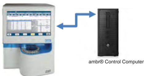
Figure 3.9 Option 1: Single network cable connecting FLEX2 to ambr®
